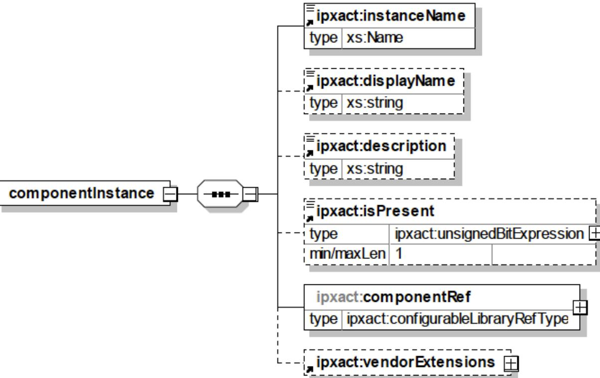
The **componentInstance** element documents the existence of a component in a design. This element contains the following subelements:
