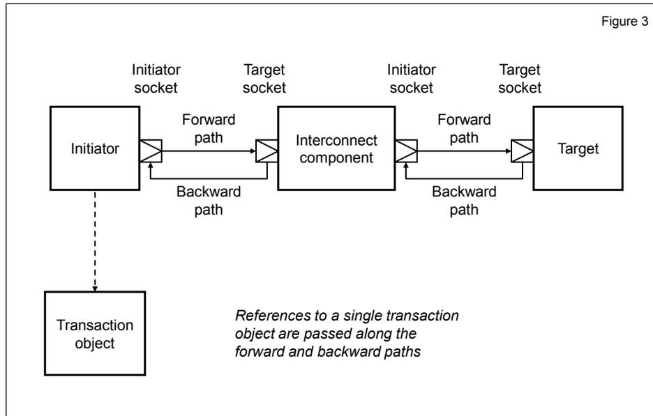
transaction, an initiator (such as a processor) writes data to a target (such as a memory). In the case of a read transaction, an initiator reads data from a target. An interconnect component is a module that accesses a
