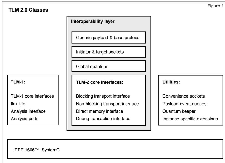
The generic payload is primarily intended for memory-mapped bus modeling, but may also be used to model other non-bus protocols with similar attributes. The attributes and phases of the generic payload can be extended to model specific protocols, but such extensions may lead to a reduction in interoperability depending on the degree of deviation from the standard non-extended generic payload.
