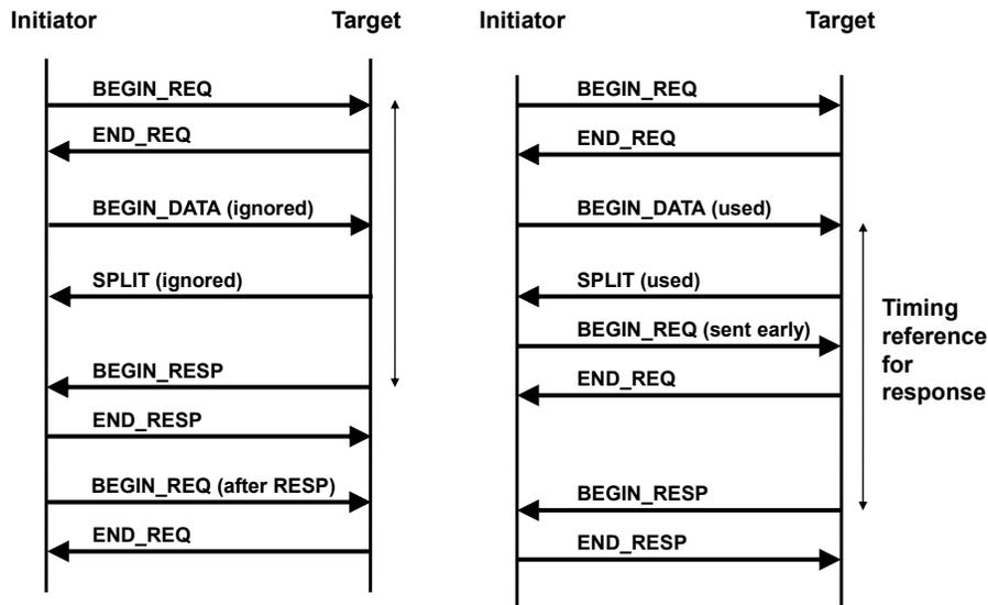
An example of an ignorable phase generated by an initiator would be a phase to mark the first beat of the data transfer from the initiator in the case of a write command. An interconnect component or target that recognized this phase could distinguish between the time at which the command and address become
