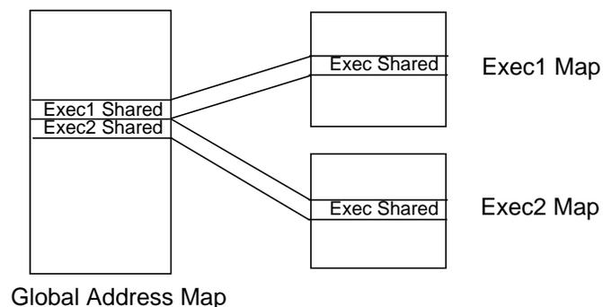
**Figure 27—Executor address mapping**
