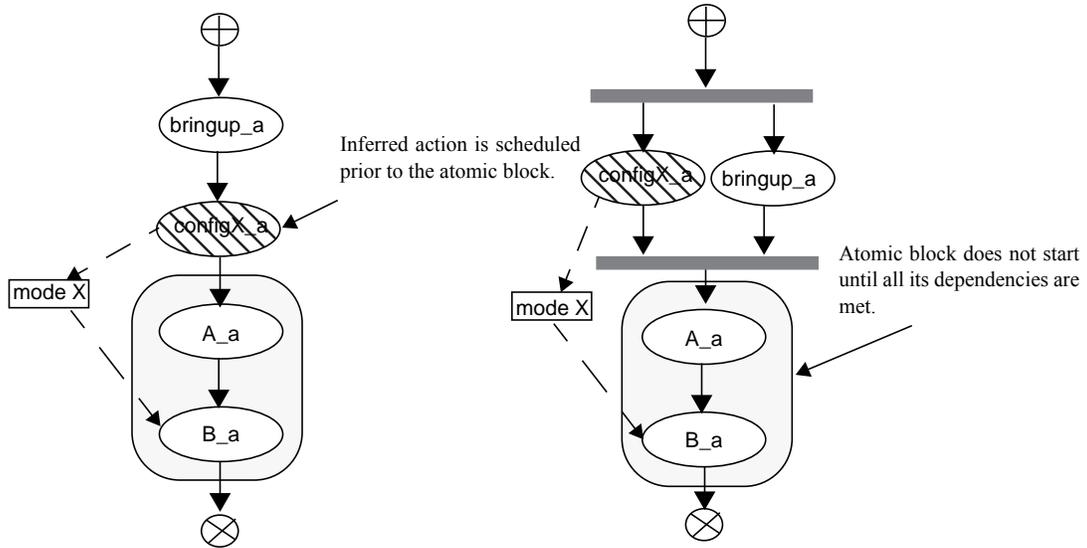
Figure 19—Scheduling graph of atomic block avoiding interference
